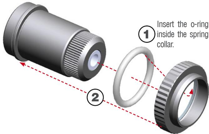
1 Insert the o-ring inside the spring collar.
