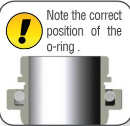
Note the correct position of the o-ring .
