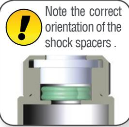
Note the correct orientation of the shock spacers .
